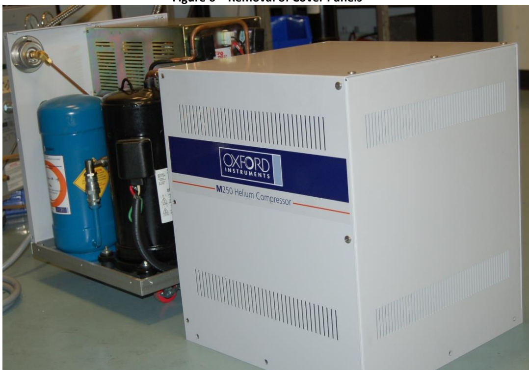
Figure 6 – Removal of Cover Panels
