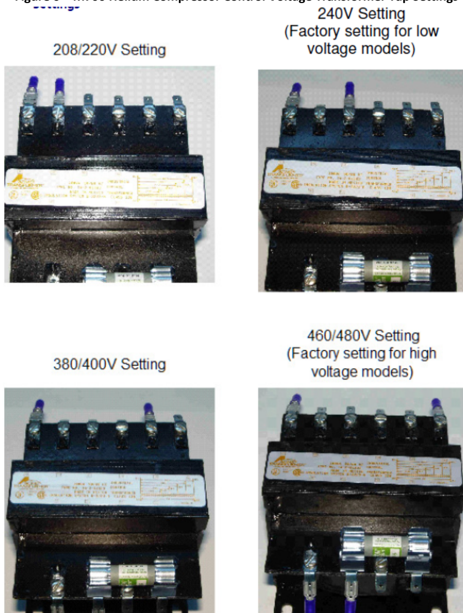
Figure 6 – M700 Helium Compressor Control Voltage Transformer Tap Settings
