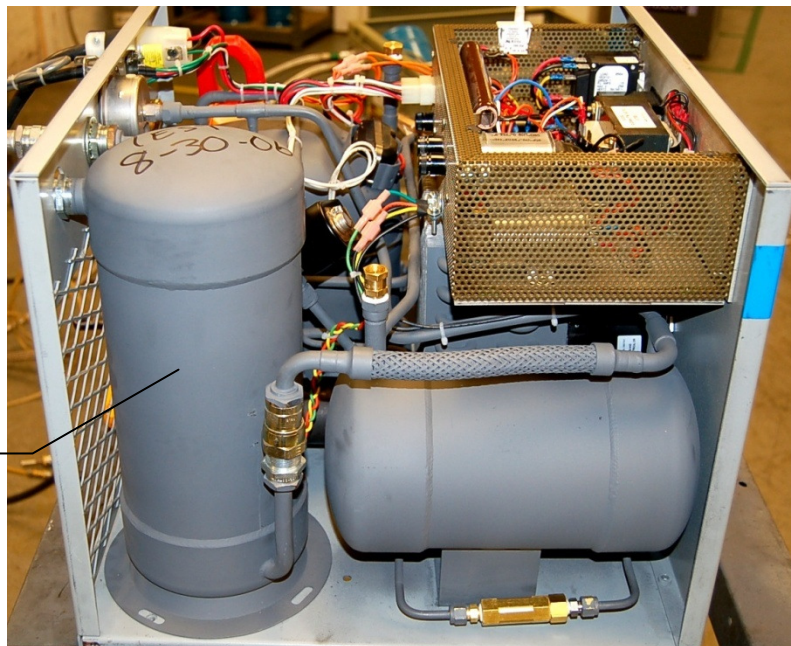
Figure 6 – Location of Adsorber in Model 125 Air-Cooled Compressor
