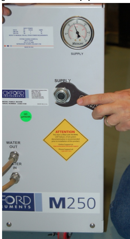
Figure 8 – Adsorber Aeroquip Nut Removal
