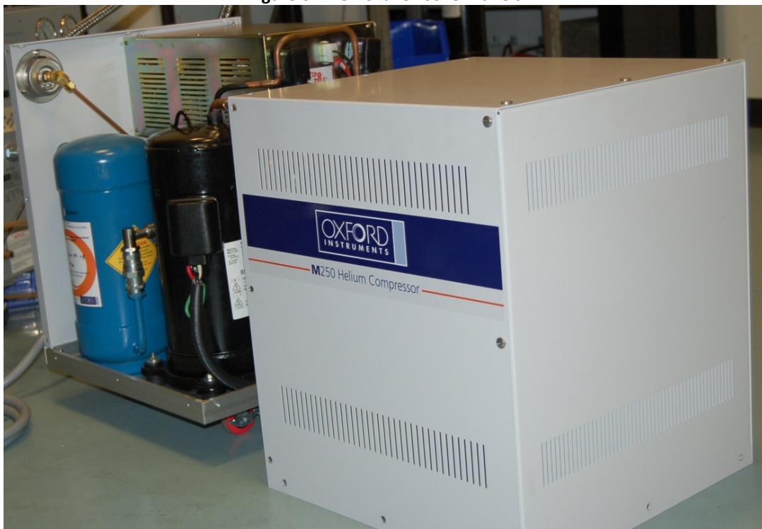
Figure 6 – Removal of Cover Panels
