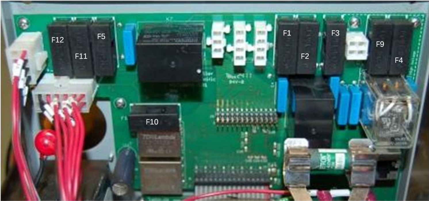
Figure 22 – M700 Fuse Locations for Electronics Boxes in Figure 2 and Figure 3
