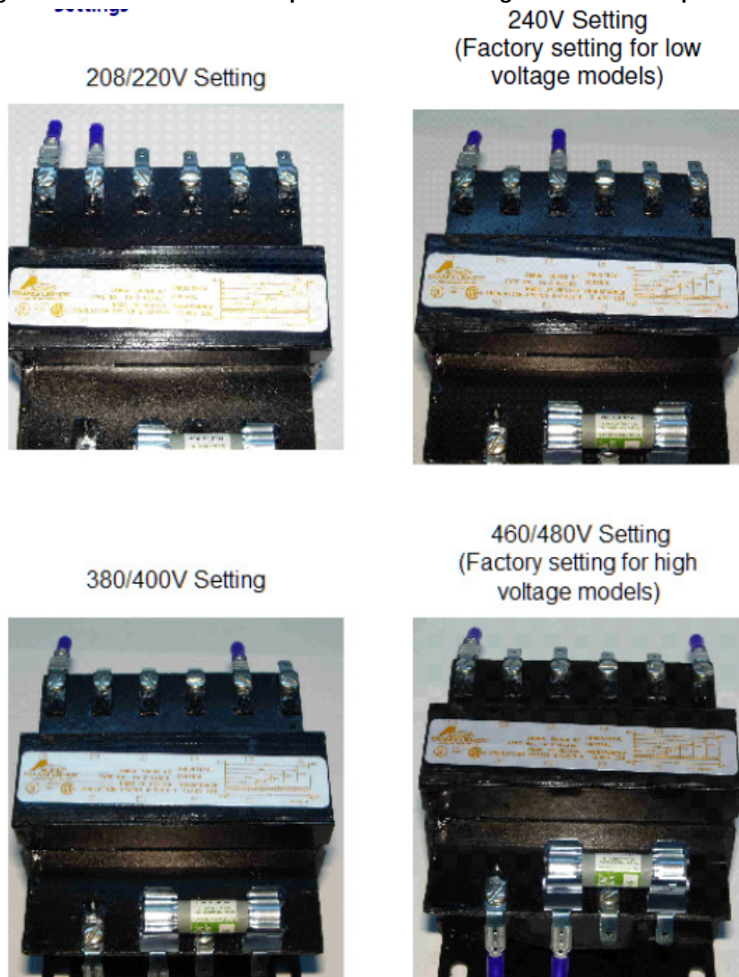
Figure 5 – M700RT Helium Compressor Control Voltage Transformer Tap Settings
