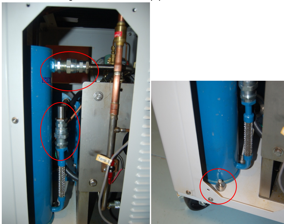
Figure 11 – Adsorber Aeroquip Connection Points
