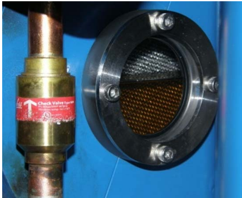
Figure 6 – Typical Sight Glass Oil Level Leaving Trillium US Inc.
